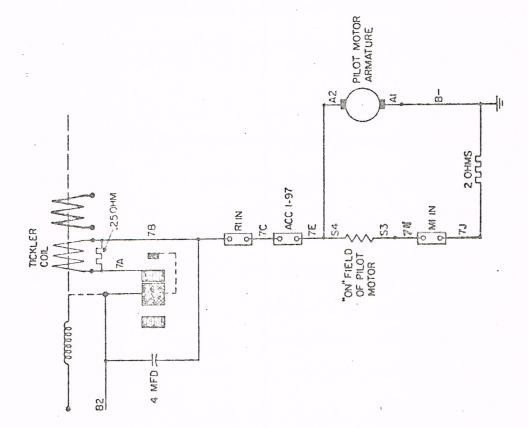
When the car operator depresses the power pedal and the R-l contactor picks up, the circuit will continue through the R-l interlock to 7C. The accelerator interlock 1-97 carries the circuit to 7E, which feeds the pilot motor.
