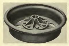
Fairmont demountable wheel of 16-in. rim can be exchanged rapidly if worn out
