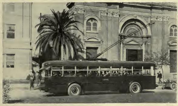
Equipped with two 50-hp. motors each, the New Orleans electric coaches are capable of attaining a maximum speed of approximately 25 m.p.h. and maintaining a schedule speed of more than 10 m.p.h.
