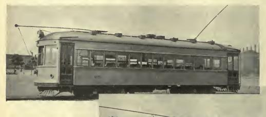
The Gary Railways Company improved local service with this type of modern light-weight car, G-E equipped
