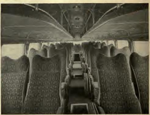
29 permanent seats with six auxiliary folding aisle chairs and tilt seat at right of driver bring total seating capacity up to 36.
