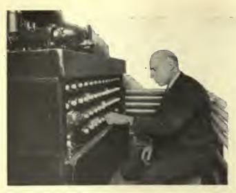
Manipulation of this switchboard by the instructor will produce symptoms of any ordinary type of electrical or mechanical
