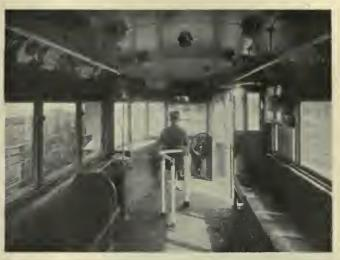
Forward platform of new Brooklyn car, showing motorman's control and arrangement of automatic turnstile at entrance to passenger well
