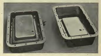
Deeper crankcase eliminates the necessity of replenishing oil supply of the bus at mid-day
