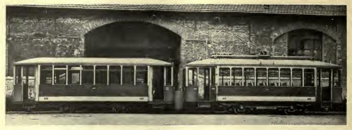
Train service consists of one motor car and trailer, both of the one-truck type. Cars in these trains have all seats facing forward
