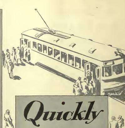
The time required to take on and discharge passengers is reduced to a minimum by NP door control equipment. Doors are opened instantly by the operator upon coming to a full stop... the operator is set to start instantly when the doors close. This saving in time with NP equipment makes possible consistently faster schedules.
