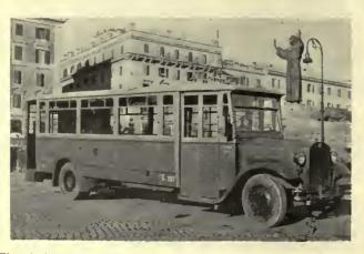
Electric buses are of the battery type and accommodate 18 seated passengers and 22 standees
