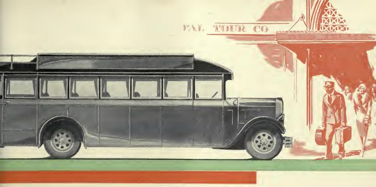
All of the excellent chassis features which made the Type W-185 coach so popular has been continued in this 215 inch chassis, with the addition of heavier construction for increased capacity.
