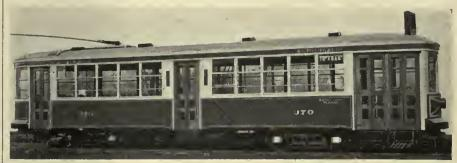
Side elevation of cars recently delivered to the British Columbia Electric Railway, showing unusual arrangement of exit doors
