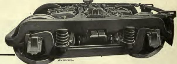
Cast steel frame, including cross and end transoms, a single strong unit.
