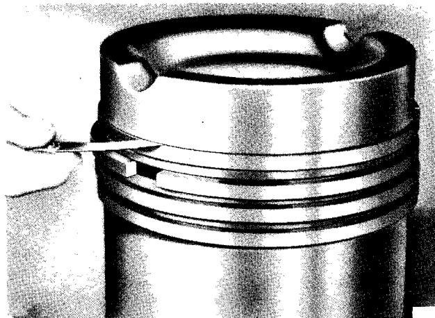
Illus. 17. Piston Ring Side Clearance
