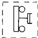
Pneumatically Operated Switch
