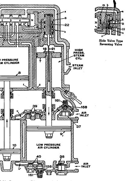
Air Compressor, Diagrammatic Section. Downward Stroke of High Pressure Steam (low pressure air) Piston
