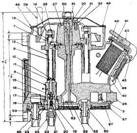
Fig. 17. Sectional Assembly Views of the "F-1-A" Lubricator
