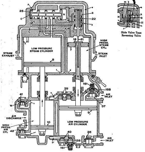
Plate 1. 81/2" Air Compressor, Diagrammatic Section. Downward Stroke of High Pressure Steam (low pressure air) Piston
