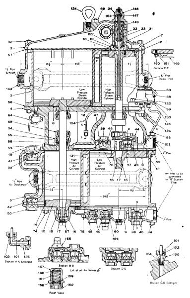
Fig. 3. Sectional View of Compressor Showing the Present Standard Piston Type Reversing Valve
