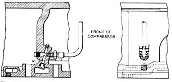
Fig. 4. Views of Center Piece, Showing Drainage and Location of Oil Hole for High Pressure Air Cylinder
