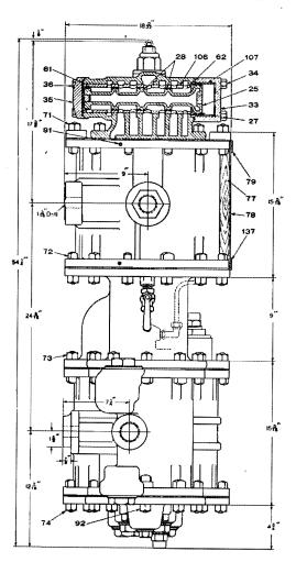
Fig. 5. Outline of Compressor with Sectional Assembly Views of the Standard Design Main Valve and Housing
