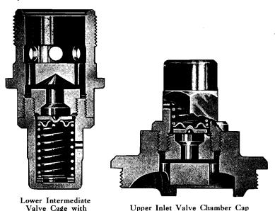
Fig. 7. Sectional Views of the Relief Valves
