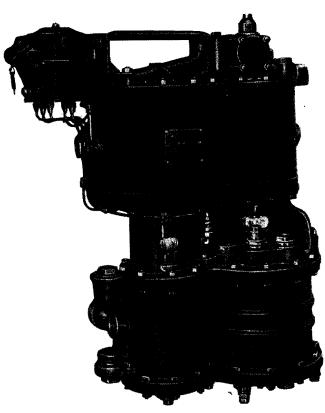
Fig. 20. Front View of the Air Compressor with the "F-1-A" Lubricator
