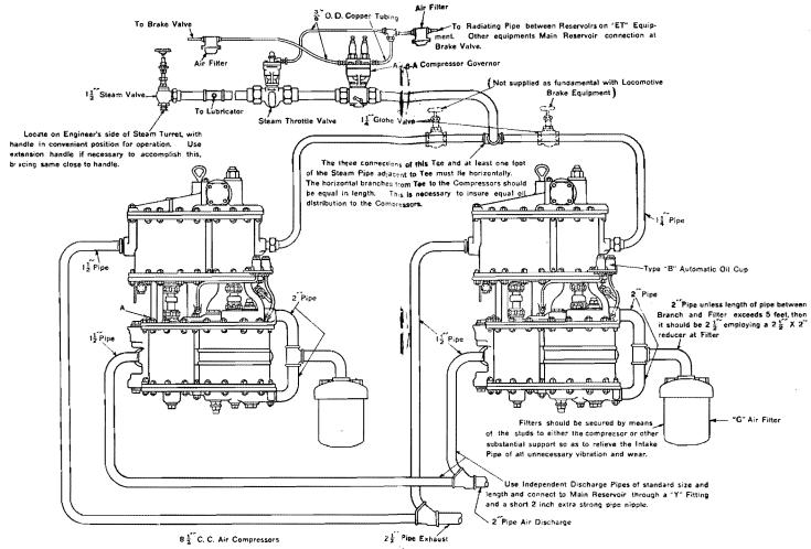
Fig. 13. Installation Diagram of Two 1/2" Cross Compound Air Compressors
